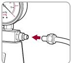
Insert PVC tubing into connector
