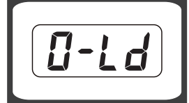
OVERLOAD INDICATION (max. weight capacity is indicated on the scale). Please step off to avoid damage.
