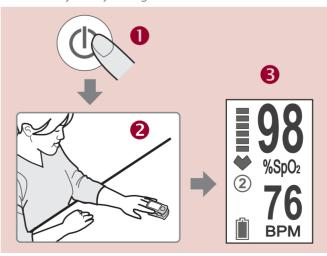
4. Your  $SpO_2$  and pulse rate values will appear on the screen after few seconds and artery check result will appear on screen after 30 - 60 seconds as 3.
